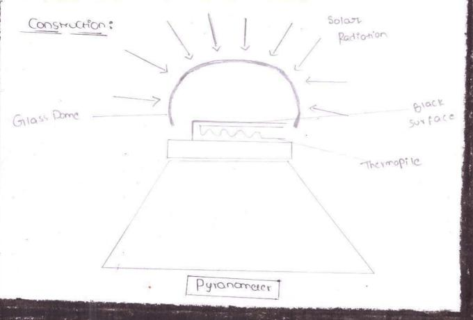
A pyranometer contain the following 3 Important parts. Black Surface: It receives the Diffuse & Direct Solar radiation. Glass Dome: It prevents the loss of radiation received by the black Surface.
